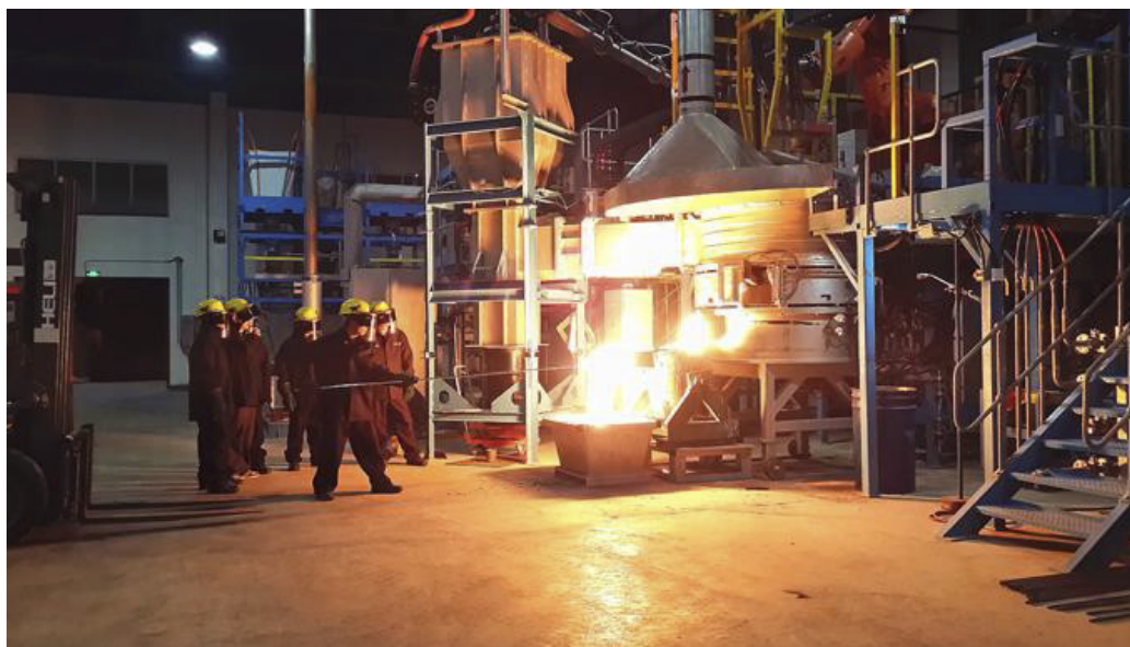
Figure 5. Commercial plasma smelting furnace for recovering platinum group metals from spent automotive catalysts at Sino-Platinum. Taken with permission from [45a].
