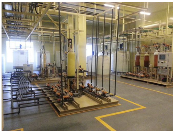
Figure 4. Commercial MRT systems for rhodium/platinum recovery at Sino-Platinum. Taken with permission from [45a].
